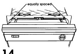
Open door approximately 3" and check for equal spacing between inner door and tub sides. If necessary, loosen screws that fasten dishwasher to countertop and shift tub. Tighten screws.
